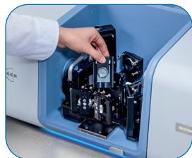
**QuickLock**, with electrical interface monitoring and its frontal one-button locking and release mechanism, ensures **faultless exchange** and **robust operation** of accessories. The automated parameter setting and verification of system performance guarantees optimal working conditions.
