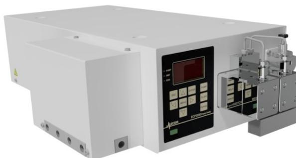
Gradient preparative pump with **four low-pressure gradient valves** and very high output pressure of **15 MPa** at flow rate up to **1000 ml/min**. It has two pistons connected in parallel, with 20 mm diameter. The pump is suited for preparative liquid chromatography where high pressure is needed, etc.
