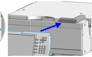
8 Connect the CAN cable of the Instant Pilot into a free CAN connector at the rear of the module.
