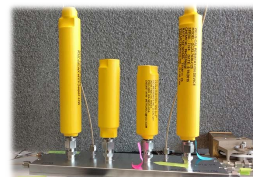
Figure 4. Permeation tubes of 4 calibrants in the dilution block.
