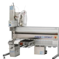
4 column set-up for automated sample clean-up in PCB and dioxin analysis
