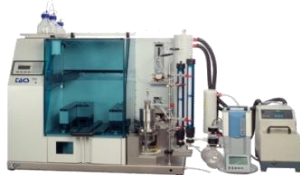
First own developed system from LCTech: TACS totally automated clean-up system for pesticide analysis
