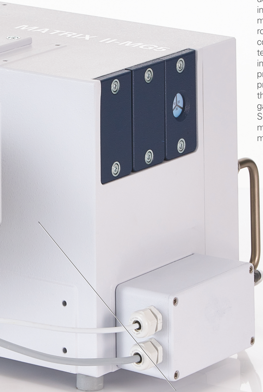
Optics compartment with IR source and RockSolid™ interferometer
