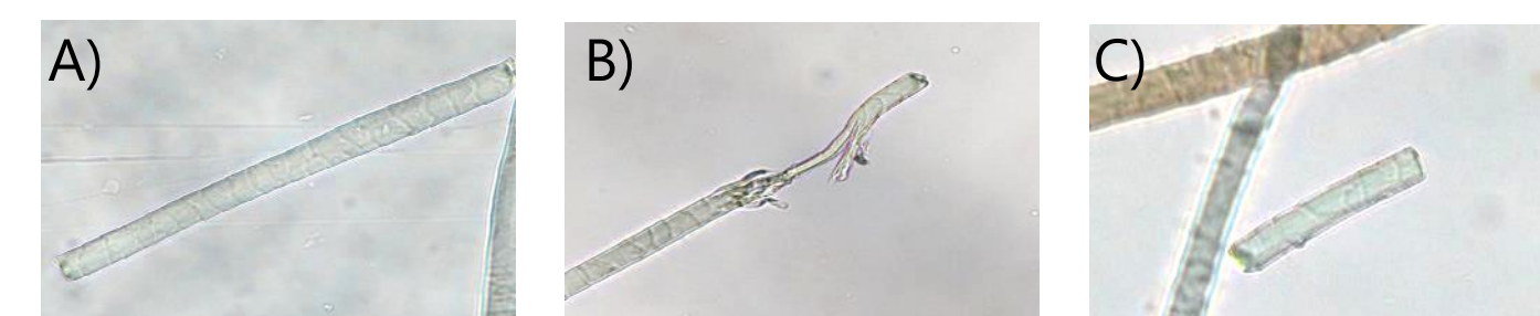
Fig. 2 Optical view of recycled cashmere fibers (x 300). A) normal, B) change of shape, C) shortened
