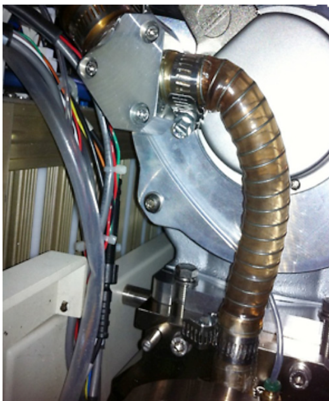
Figure 2 – Discoloration of Foreline Tubing from RVP
