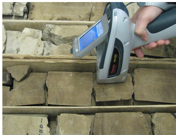
Figure 1. Rapid elemental analysis by handheld XRF and elemental ratio plots is a valuable tool in well logging and exploration.
