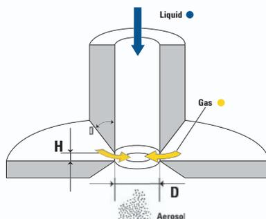
The Flow Blurring nozzle configuration promotes highly turbulent mixing between the liquid sample and the nebulizer gas flow – creating a fine aerosol of extremely small droplets.
