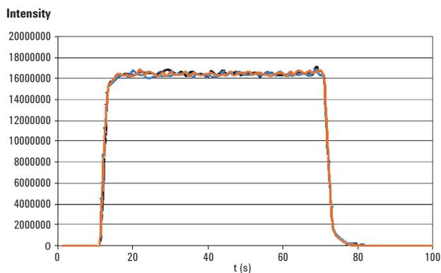
Washout profile for 25 ppm Mn in 1% nitric acid using the single-pass glass cyclonic spray chamber (3 replicates).
