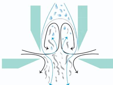
Turbulent mixing between a liquid (blue) and gas (black).
