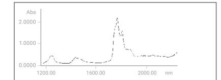
These two scans demonstrate the effect of varying the SBW The above graph shows a scan of hexane with a SBW of 15 nm.
