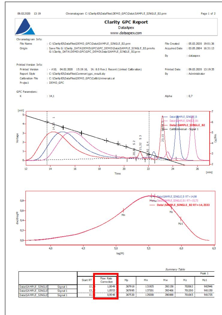
→ Flow rate correction applied in the second chromatogram
