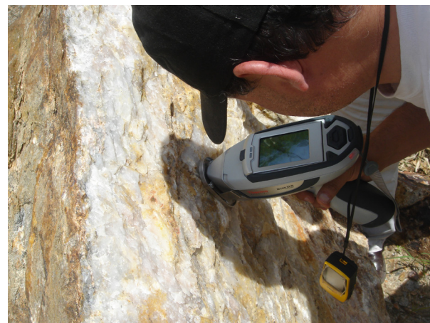
Thermo Scientific portable XRF analyzers deliver fast and accurate analysis of pathfinder elements for precious metal exploration.
