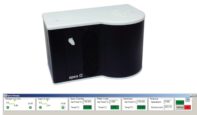
FIGURE 1. Image of Elemental Scientific apex \Omega and screenshot showing software control for precise gas tuning.
