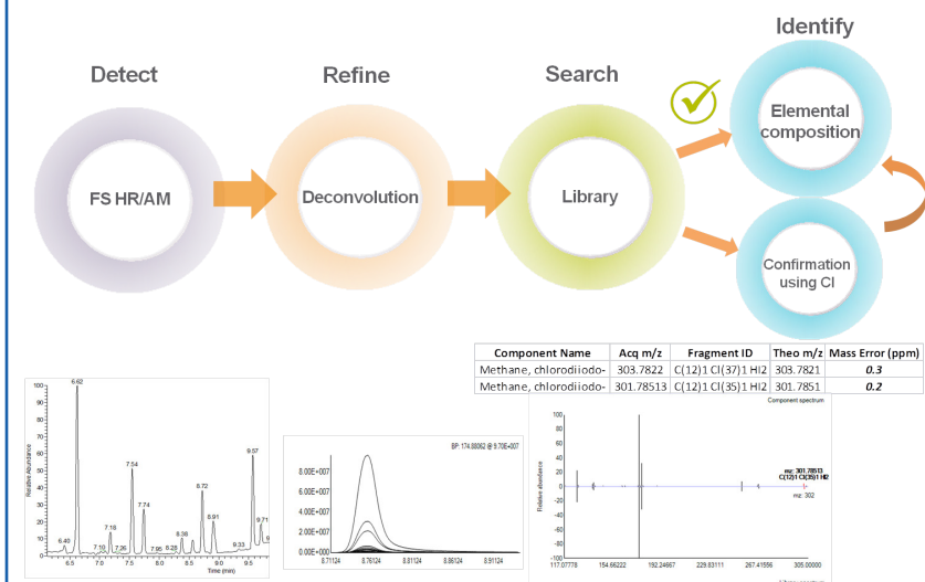
Figure 2. Compound discovery workflow used for iodo-DBP peak detection with spectral deconvolution and tentative compound identification
