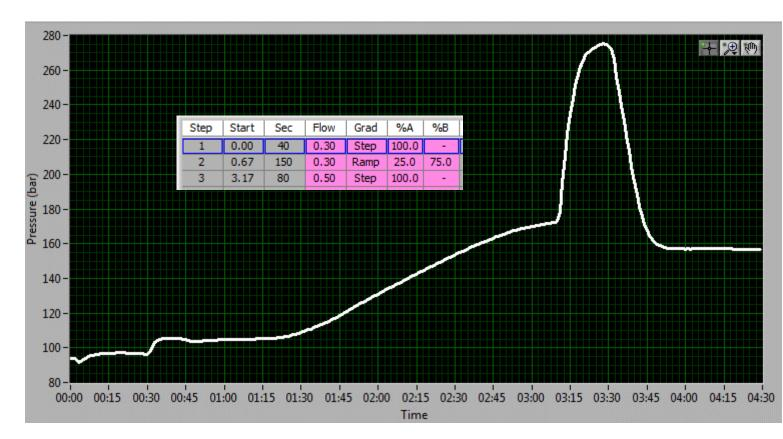
Figure 4. Autosampler method with air gap and organic needle wash parameters that remedied peak-shape problems.
