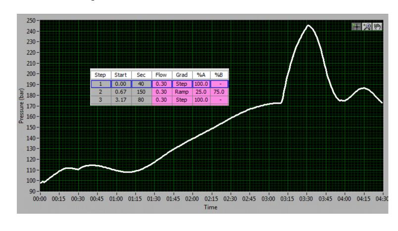
Figure 3. PFP column pressure trace showing sufficient equilibration.
