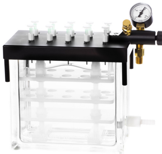
Figure 12. Vacuum manifold for manual processing of SPE columns.
