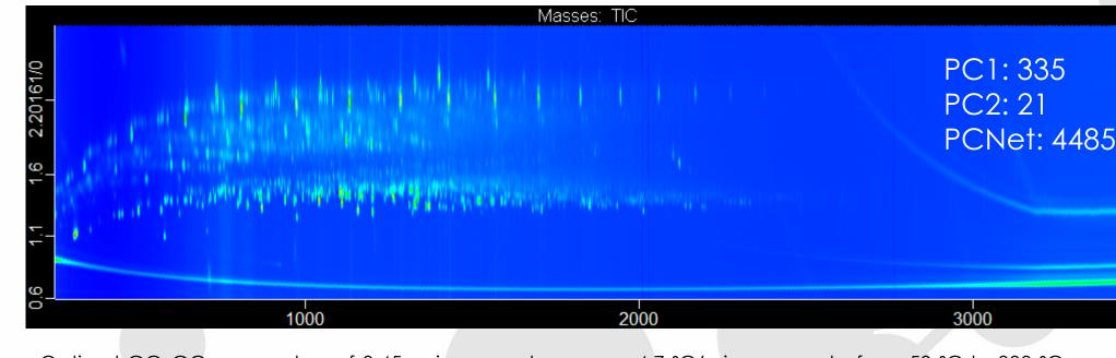
Optimal GCxGC parameters of 0.45 m in secondary oven, 4.7 °C/min ramp rate from 50 °C to 300 °C, carrier gas flow rate of 1.4 mL/min, +9 °C secondary oven offset, 2<sup>nd</sup> dimension separation time of 2.2 s with 0.65 s hot pulse, and spectral acquisition rate of 248 spectra/s. Total peak capacity calculated at 4485.
