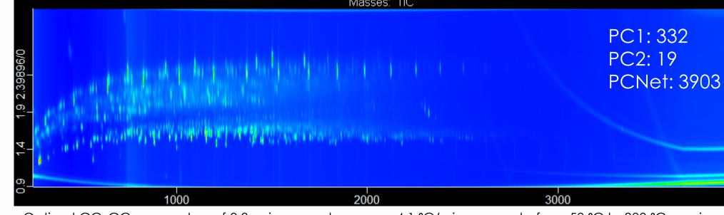
Optimal GCxGC parameters of 0.3 m in secondary oven, 4.1 °C/min ramp rate from 50 °C to 300 °C, carrier gas flow rate of 1.4 mL/min, +9 °C secondary oven offset, 2<sup>nd</sup> dimension separation time of 2.4 s with 0.73 s hot pulse, and spectral acquisition rate of 193 spectra/s. Total peak capacity calculated at 3903.
