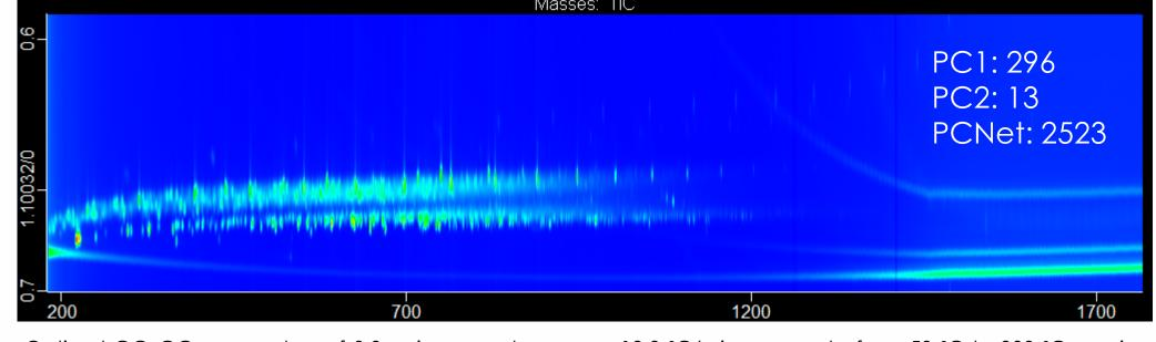
Optimal GCxGC parameters of 0.3 m in secondary oven, 10.3 °C/min ramp rate from 50 °C to 300 °C, carrier aas flow rate of 1.4 mL/min, +32 °C secondary oven offset, 2<sup>nd</sup> dimension separation time of 1.1 s with 0.33 s hot pulse, and spectral acquisition rate of 309 spectra/s. Total peak capacity calculated at 2523
