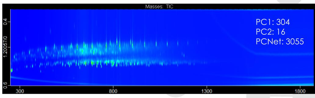
Optimal GCxGC parameters of 0.45 m in secondary oven, 9.6 °C/min ramp rate from 50 °C to 300 °C, carrier gas flow rate of 1.4 mL/min, +9 °C secondary oven offset, 2<sup>nd</sup> dimension separation time of 1.2 s with 0.30 s hot pulse, and spectral acquisition rate of 349 spectra/s. Total peak capacity calculated at 3055.
