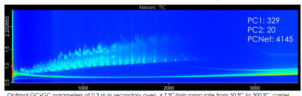
Optimal GCxGC parameters of 0.3 m in secondary oven, 4.7 °C/min ramp rate from 50 °C to 300 °C, carrier gas flow rate of 1.4 mL/min, +10 °C secondary oven offset, 2<sup>nd</sup> dimension separation time of 2.2 s with 0.60 s hot pulse, and spectral acquisition rate of 234 spectra/s. Total peak capacity calculated at 4145.
