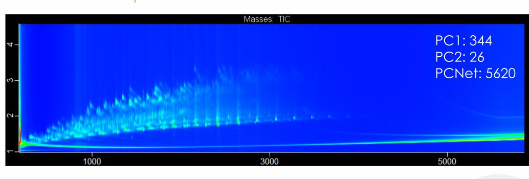
Optimal GCxGC parameters of 0.45 m in secondary oven, 2.7 °C/min ramp rate from 50 °C to 300 °C, carrier gas flow rate of 1.4 mL/min, +15 °C secondary oven offset, 2<sup>nd</sup> dimension separation time of 3.6 s with 1.10 s hot pulse, and spectral acquisition rate of 178 spectra/s. Total peak capacity calculated at 5620.
