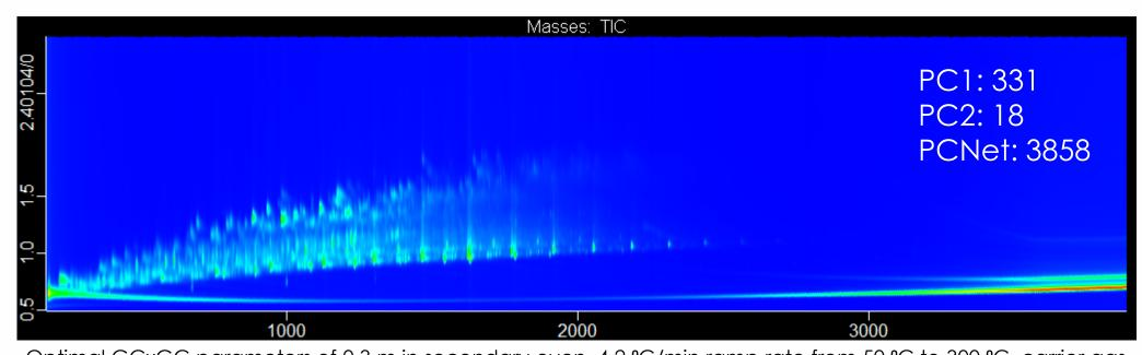
flow rate of 1.4 mL/min, +9 °C secondary oven offset, 2<sup>nd</sup> dimension separation time of 2.4 s with 0.73 s hot pulse, and spectral acquisition rate of 192 spectra/s. Total peak capacity calculated at 3858.
