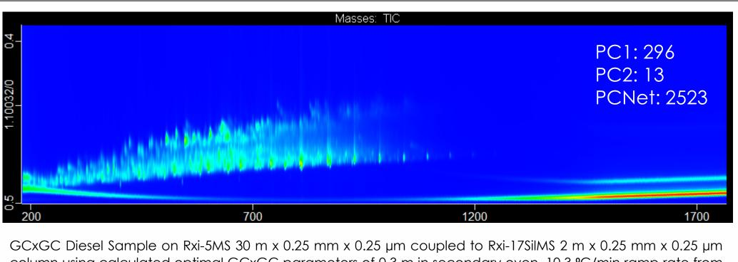
column using calculated optimal GCxGC parameters of 0.3 m in secondary oven, 10.3 °C/min ramp rate from 50 °C to 300 °C, carrier gas flow rate of 1.4 mL/min, +16 °C secondary oven offset, 2<sup>nd</sup> dimension separation time of 1.1 s with 0.33 s hot pulse, and spectral acquisition rate of 309 spectra/s.
