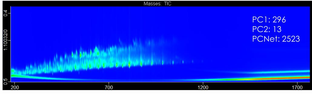
Optimal GCxGC parameters of 0.3 m in secondary oven, 10.3 °C/min ramp rate from 50 °C to 300 °C. carries gas flow rate of 1.4 mL/min, +16 °C secondary oven offset, 2<sup>nd</sup> dimension separation time of 1.1 s with 0.33 s hot pulse, and spectral acquisition rate of 309 spectra/s. Total peak capacity calculated at 2523
