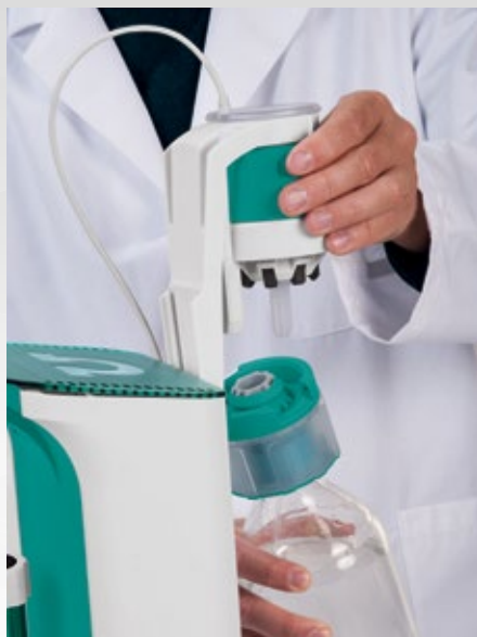
▲ Fig. 3: More safety and reliability: Reagents for the new titration platform come in bottles with an RFID chip in their cap. As soon as this cap is connected to the Omnis Titrator with the new Omnis Liquid Adapter, the system identifies and checks the reagent against the specifications of the method to be performed.
