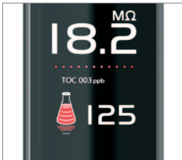
Figure 4: ELGA PURELAB Chorus 1 with Halo Dispense display showing TOC reading
