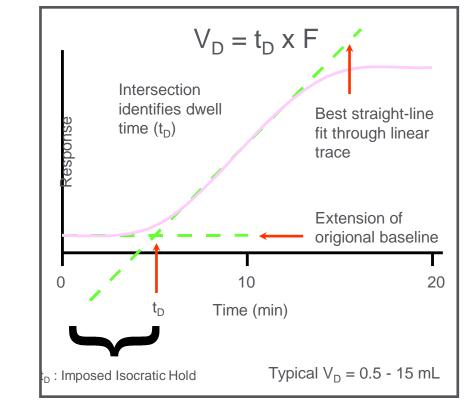
High Pressure Mixing:  $V_D$  = mixing chamber + connecting tubing + injector Low Pressure Mixing:  $V_D$  = the above + pump heads + associated plumbing
