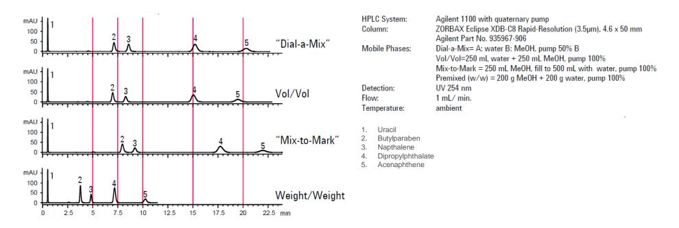
Method used to prepare MP can significantly affect the elution pattern
