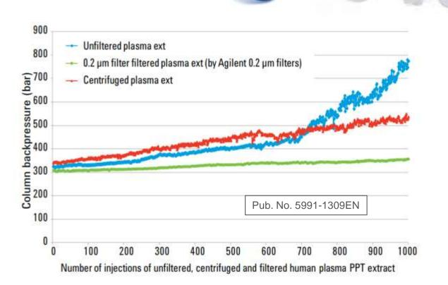
Unfiltered, centrifuged, and filtered plasma extracts Zorbax RRHD Eclipse Plus C18, 2.1 x 50 mm, 1.8 µm column, PN 959757-902
