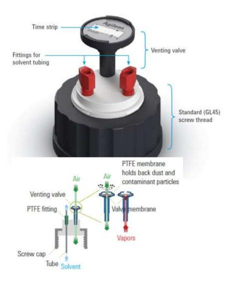
The venting valve plays an important role in maintaining your workspace, keeping it safe and clean. It blocks harmful vapors and assures the required ventilation while solvent is being pulled to the LC instrument.
