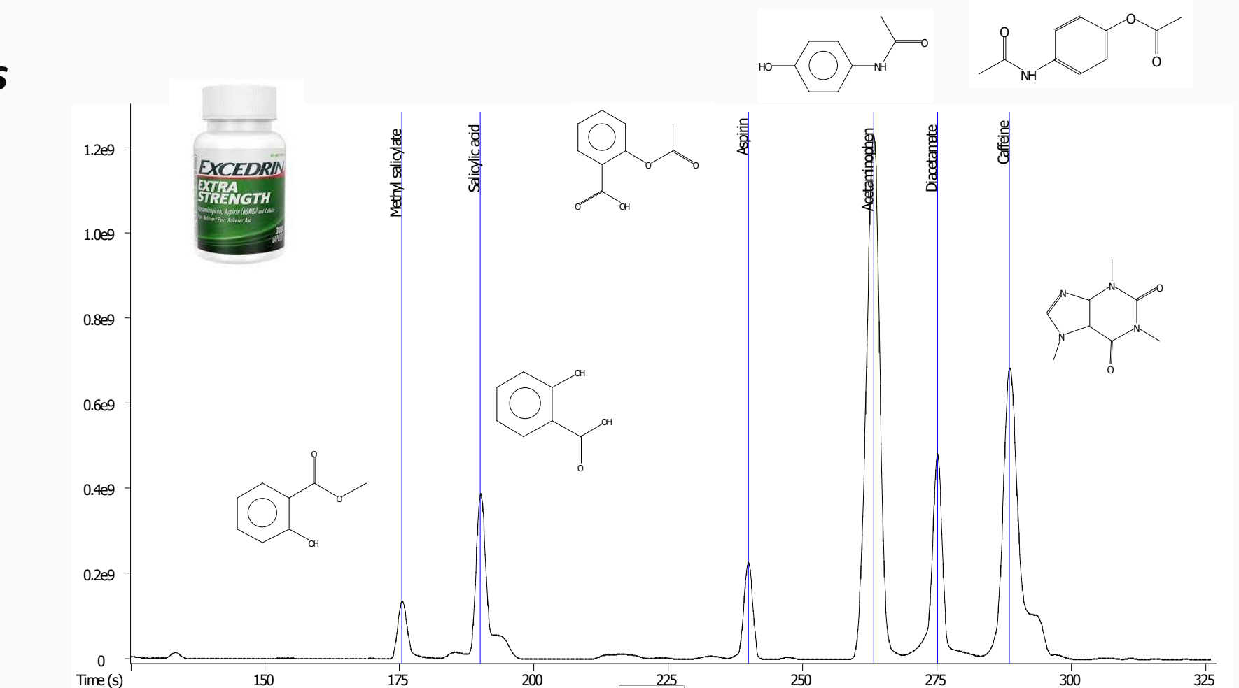
Figure 10: Analytical Ion Chromatogram Showing Selected Excedrin Constituents
