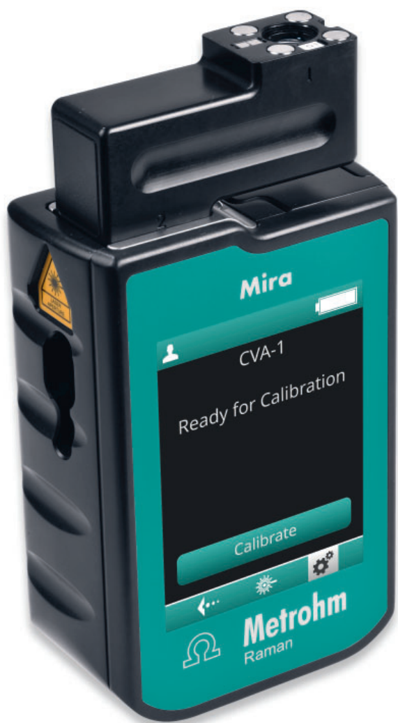
Figure 4: Mira P with Calibrate/Verify Accessory
