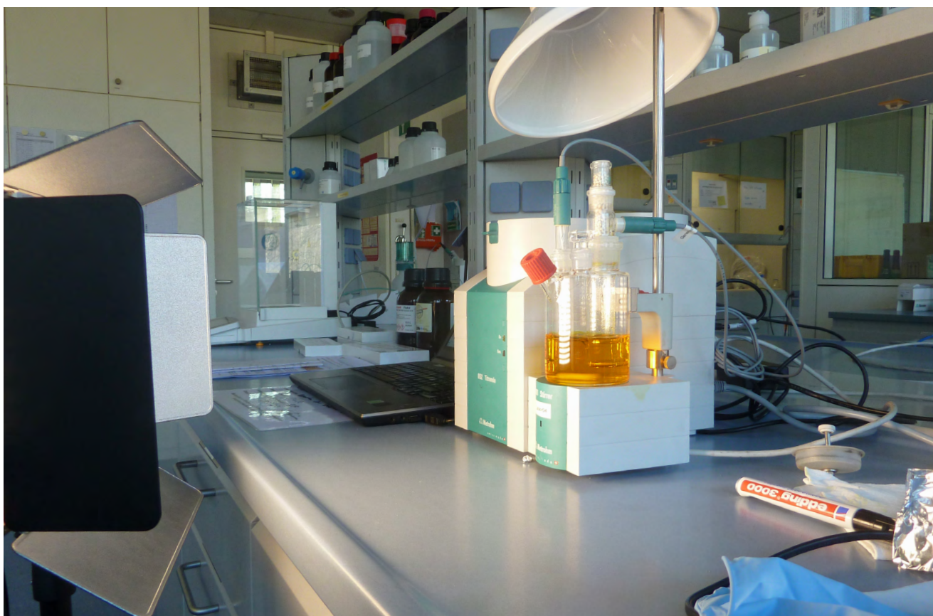
Figure 3. Experimental setup to study the photosensitivity of the Hydranal alcohol-free KF reagents.
