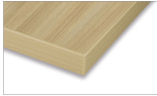
25 mm work surface 0.8 mm HPL coated oak, 3 mm PP edge oak
