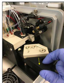
Place ZipChip and prepare the system
