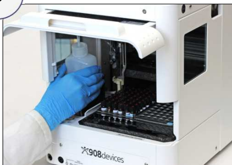
Place ZipChip and prepare the system
