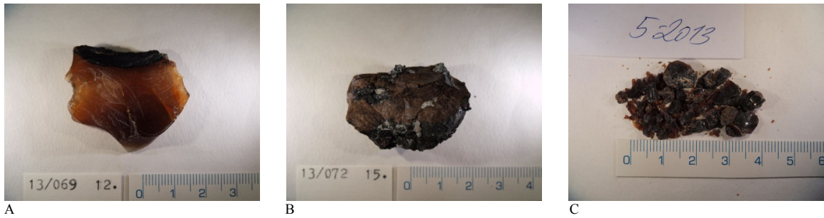
Fig. 2. Photomicrographs of resinite occurrences: brown and partly transparent resin - Sarawak amber (A); brown opaque resin - Krizany (B); brown, partly transparent, resinous gloss - Duxite (C).
