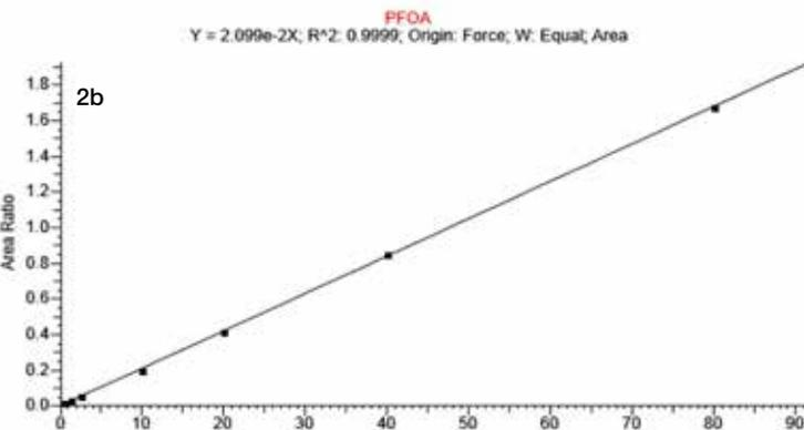
Figure 5. Comparison of full scan extracted ion and PRM scan modes for the compound PFOA at 0.5 ppt and calibration linearity from 0.5 to 80 ppt. (1a, 1b) PRM with primary MS2 transition used for quantitation; (2a, 2b) Full scan extracted ion at 70,000 FWHM used for quantitation.
