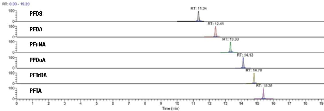
Figure 4. Full scan extracted ion chromatogram of target compounds at 70K resolution, showing good peak shapes and S/N for a 2.5 ppt standard.
