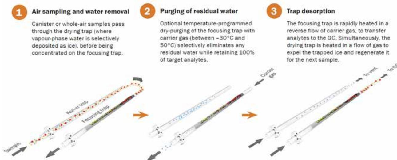
Figure 5. Operation of Dry-Focus3. For an example of the use of trap dry-purging, see Markes Application Note 133.<sup>6</sup>
