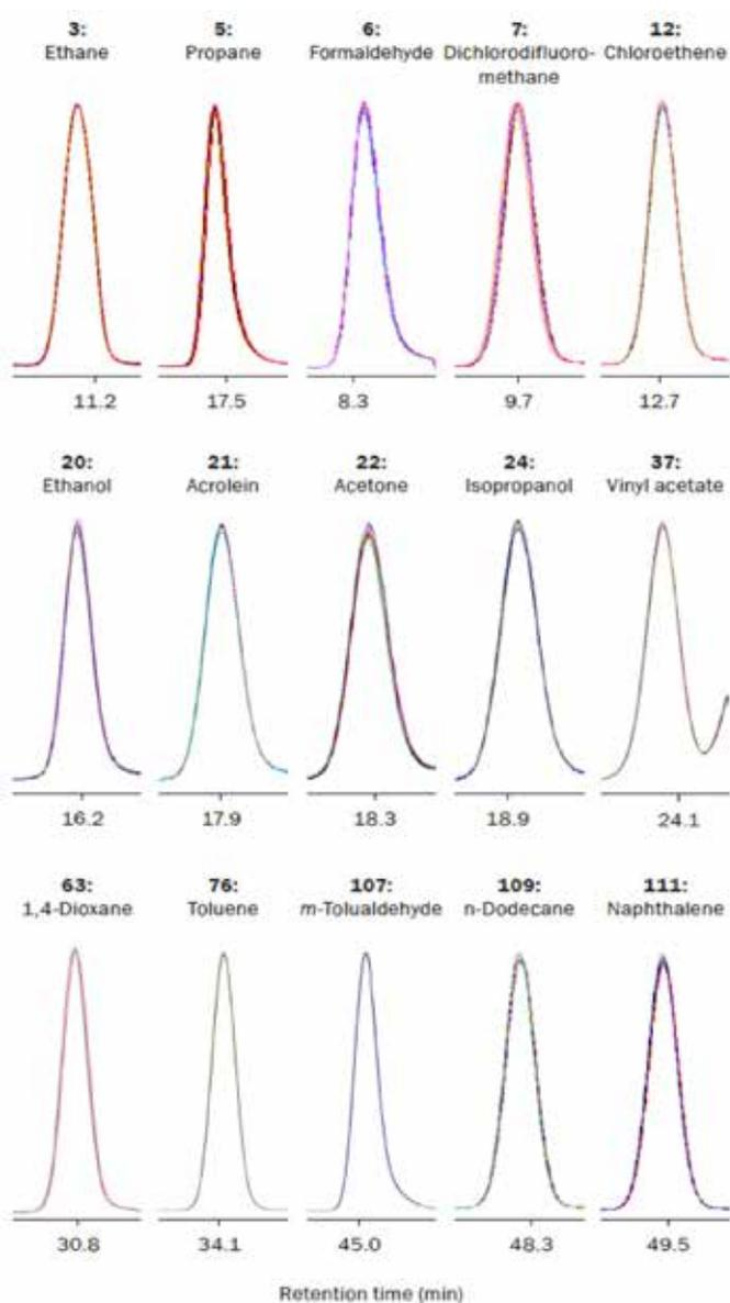
**Figure 9. Example overlaid responses (FID for ethane and propane, MS SIM for formaldehyde, MS EIC otherwise) for ten repeat analyses of 400 mL of the 10 ppb, 100% RH standard, demonstrating excellent retention time and response stability**
