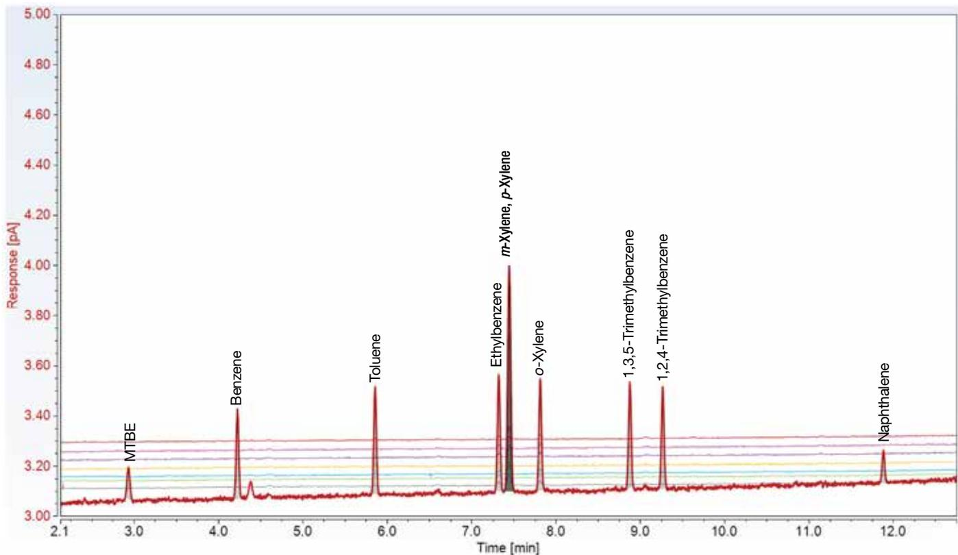
Figure 2. Comparison between chromatograms obtained analyzing  $n = 7$  real tap water samples (unspiked) and a tap water sample spiked at  $12.5 \mu\text{g/L}$  (ppb) (red trace). None of the investigated gasoline organics could be detected in the unspiked tap water samples.
