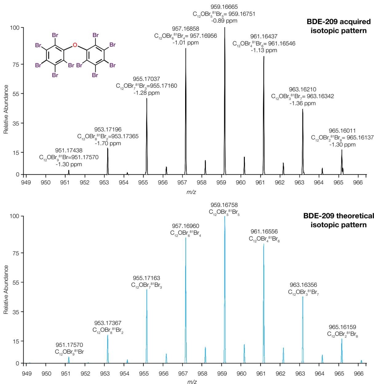
**Figure 5. Comparison of mass spectra for BDE-209, acquired isotopic pattern (upper) versus the theoretical isotopic pattern (lower).** Consistent <2 ppm mass accuracy obtained for each of the ion in the cluster. Annotated are the measured mass, the elemental composition, and the theoretical mass as well as the mass accuracy (ppm).
