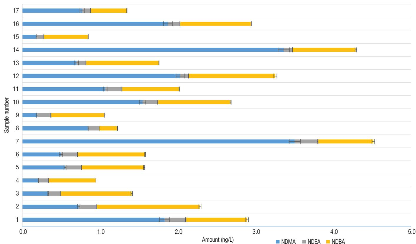
**Figure 7. Total quantified nitrosamine content (ng/L) from 17 drinking water samples sourced from separate water testing facilities across Europe.** NDMA d-6 and NDEA d-10 surrogate standards were spiked to 1 L of water pre-extraction at 25 ng/L to correct recoveries for NDMA and NDEA. Deuterated NDBA was not available for the analysis so the values are not corrected. The mean and standard deviation for triplicate injections per sample are presented in the chart.
