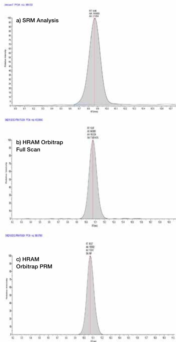
**Figure 6. A 2.5 ppt standard of PFOA analyzed by both Q Exactive MS and triple quadrupole mass analyzers under similar conditions (all 5  $\mu$ L injections). Excellent quantitation and sensitivity is obtained with HRAM Orbitrap in comparison to QQQ analysis.**
