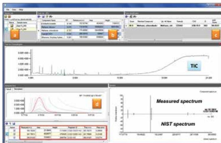
Figure 3. Deconvolution browser showing chlorodiiodomethane identification based on library (NIST) match search index, SI 963), fragment rationalization with an HRF > 99% and mass accuracies of measured fragments (e.g., molecular ion  $m/z$  301.78513 ppm = 0.23). Samples processed (a), peaks detected (b), identified chemicals (c), and deconvoluted mass spectra for chlorodiiodomethane (d) with the measured and theoretical ions including mass errors are indicated.
