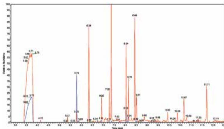
Figure 1. Overlaid extracted ion chromatograms ( $m/z$  126.90392, iodine) of Milli-Q water spiked with natural organic matter (NL NOM) subjected to chlorination (red) and control of untreated water (blue) showing an increase in both the number and intensity of iodine-containing peaks in the chlorinated water as compared to the control.
