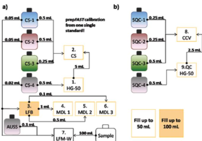
AUSS: Gold Standard Solution, CCV: Continuous Calibration Verification, CS-1 to 4: Calibration Standards, HG-50: Mercury Standard (50 ppb), LFB: Laboratory Fortified Blank, LFM-W: Laboratory Fortified Matrix, MDL-1 to 3: Solutions to determine Method Detection Limit, SQC-1 to 4: Standards for Quality control.
