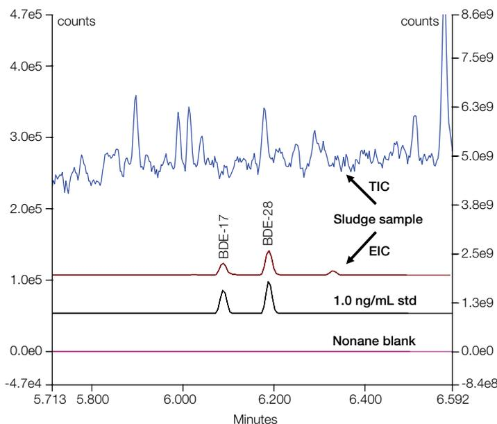
**Figure 11. Overlaid EICs for BDE-17 and BDE-28 (left), in 1.0 ng/mL standard, an extracted sludge sample at a similar level, and a nonane blank. In addition, the TIC for the extracted sludge sample (right).**
