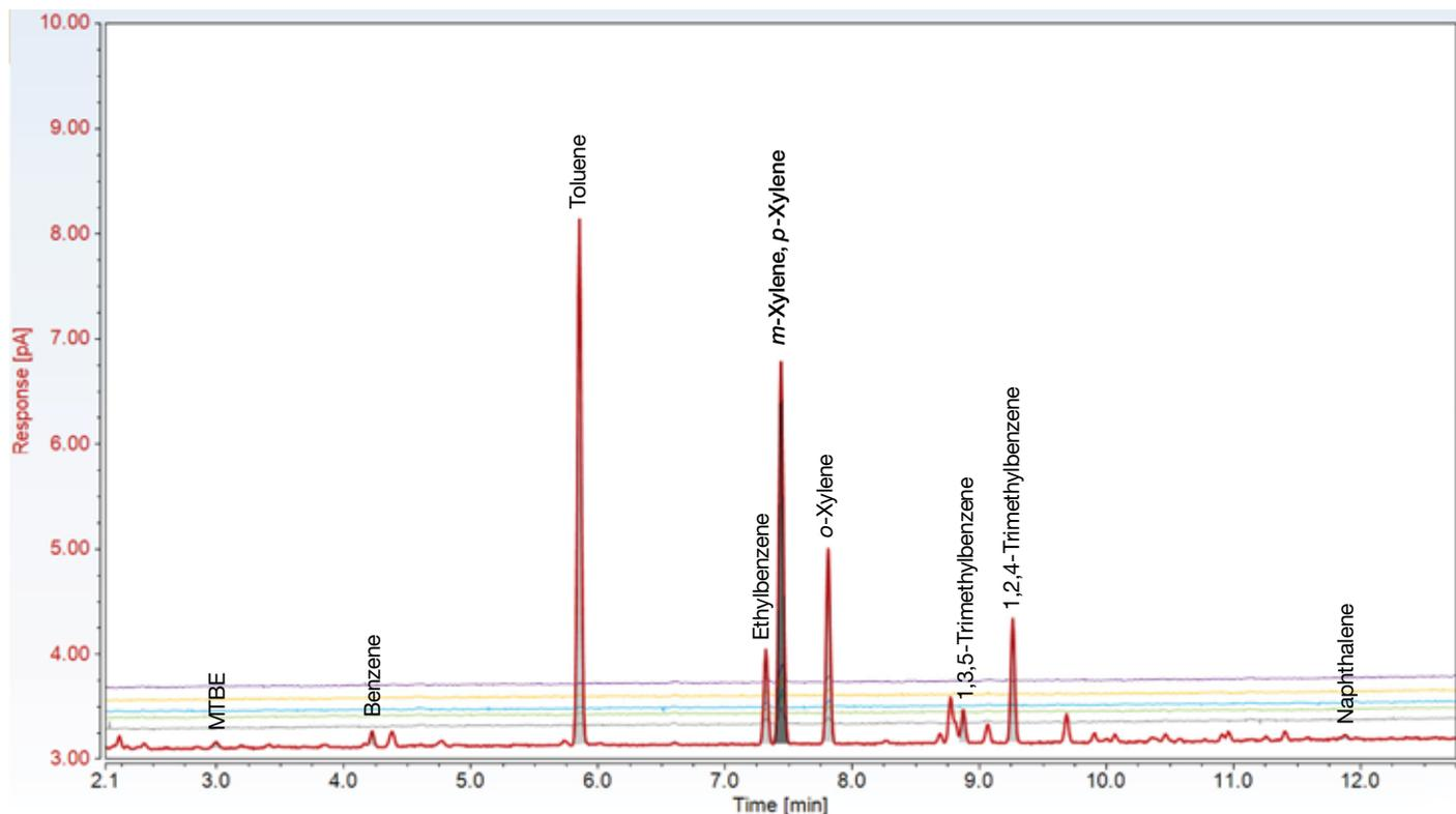
Figure 5. Comparison between chromatograms obtained analyzing  $n = 5$  blank water vials after completing the sample sequence and a sample spiked with  $1 \mu\text{L}$  of raw gasoline solution (5%) (red trace). None of the investigated gasoline organics or any residual matrix components could be detected in the blank water.
