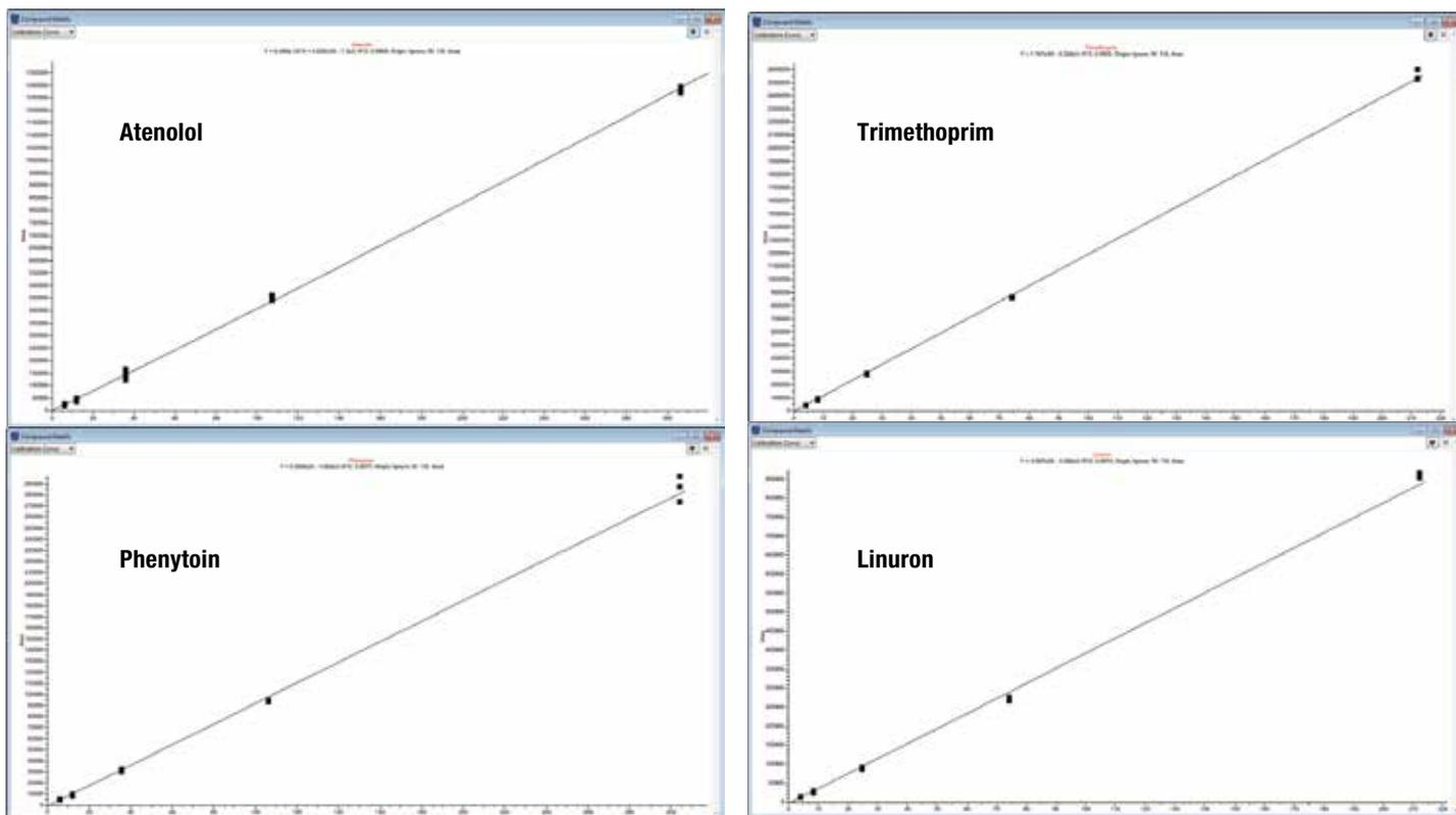
Figure 4. Standard calibration curves for positive ion compounds.
