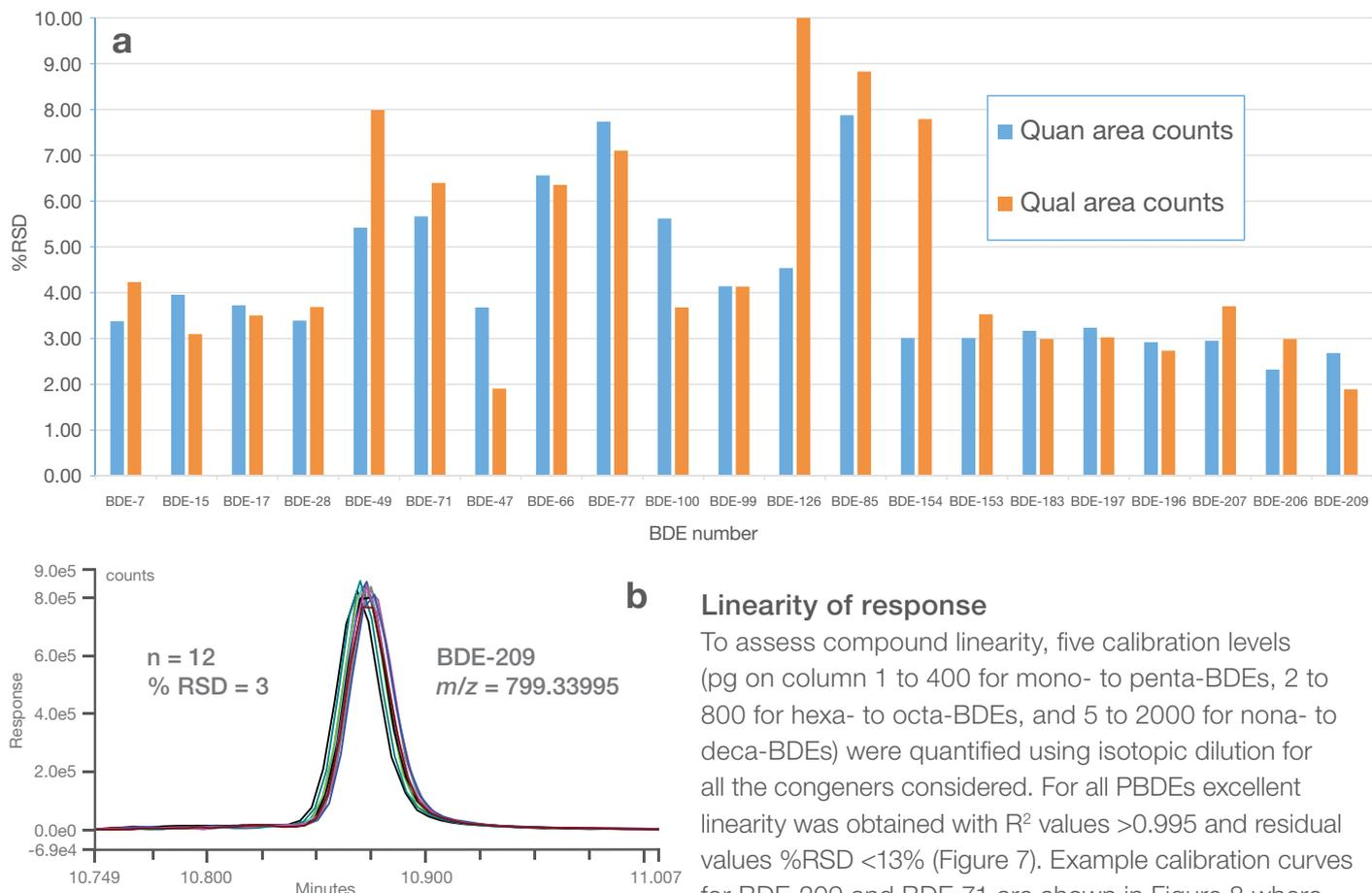
Figure 6. Replicate injections (n=12) of a filter dust sample, a) quantification and qualification area counts %RSD values for identified congeners, b) overlaid EICs ( $m/z$  799.33995) for BDE-209
