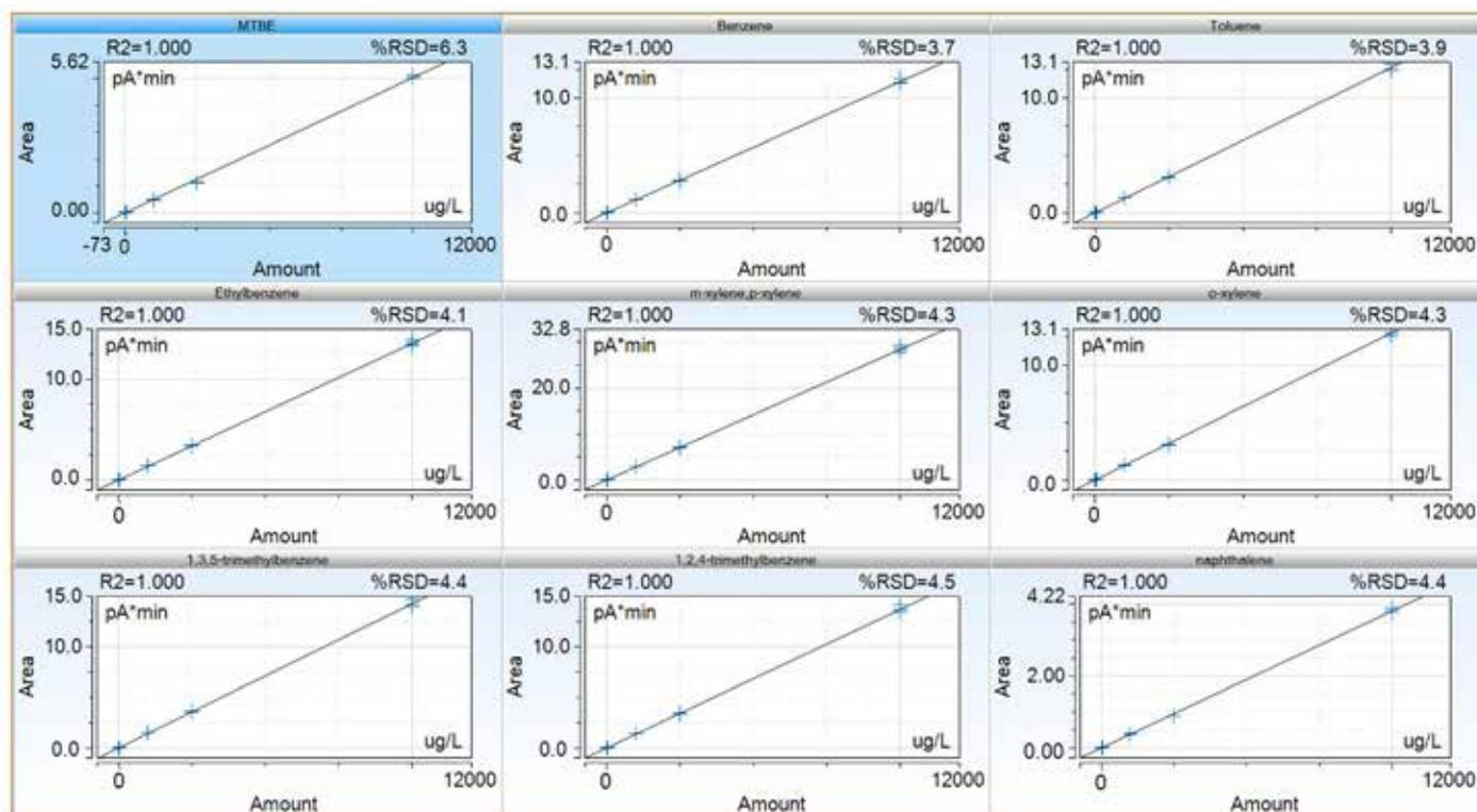
Figure 1. Calibration curves for GRO obtained by injecting seven concentration levels (6.25 to 10,000 µg/L). R<sup>2</sup> as well as response factors relative standard deviations (% RSD) are shown. Each calibration level was prepared and analyzed in triplicate (n = 3).
