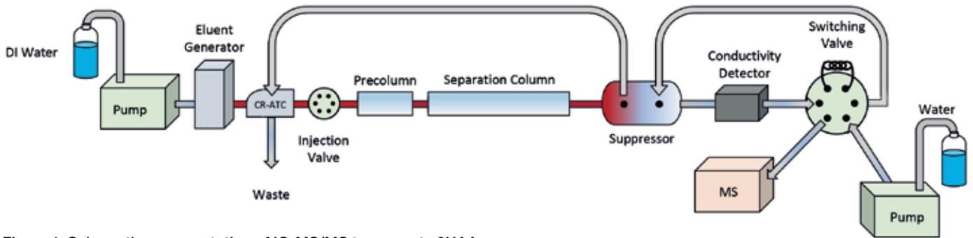
Figure 1. Schematic representation of IC-MS/MS to separate 9HAA
