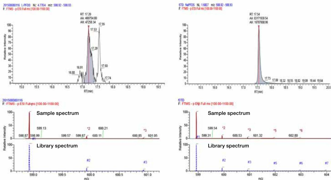
**Figure 10. A UCMR3 sample shown having trace hits for a non-targeted compound (PFDS).** Post-run identification was performed using an in-house spectral library with isotopic pattern recognition, accurate mass, and retention time for confirmation.
