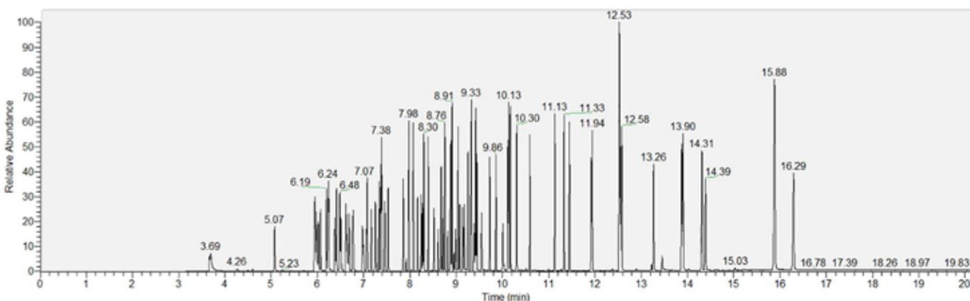
Figure 2. Total ion current (TIC) chromatogram of the 5 ppm EPA 8270 semivolatile calibration standard injected in splitless mode.
