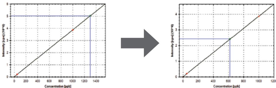
Analytes exceeding the calibration curve trigger the intelligent auto-dilution!
