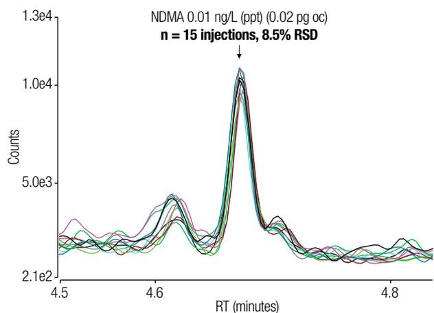
**Figure 4. Overlaid quantification SRM transitions (74 → 44 m/z) from n=15 consecutive injections of a 0.01 pg/μL NDMA solvent standard corresponding to 0.01 ng/L in sample. No data smoothing was used and data was acquired in timed-SRM mode.**
