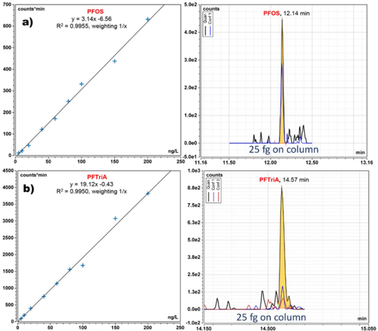
Figure 2. Representative calibration curves for a) PFOS and b) PFTriA, and chromatograms of an injection of 1 ng/L, which is five times lower than the reporting limit of quantitation
