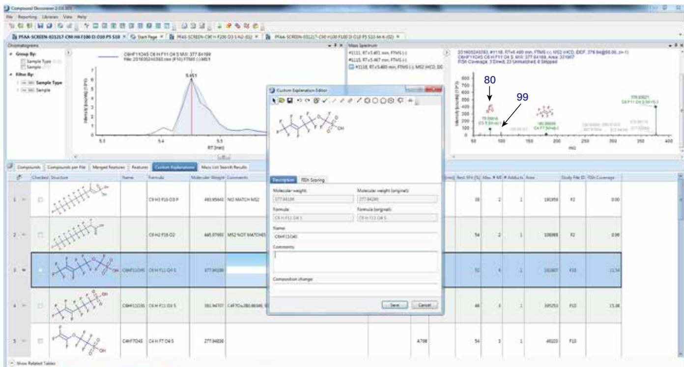
**Figure 12. A proposed structure can be drawn in a ‘custom explanations’ window in Compound Discoverer software using Mass Frontier software for FISH coverage and to check against accurate mass, isotope pattern, with MS2 data displayed in the same workspace.**
