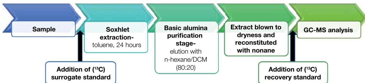
Figure 2. PBDE analytical workflow, including sample extraction, extract purification, and concentration stages required prior to GC-MS analysis
