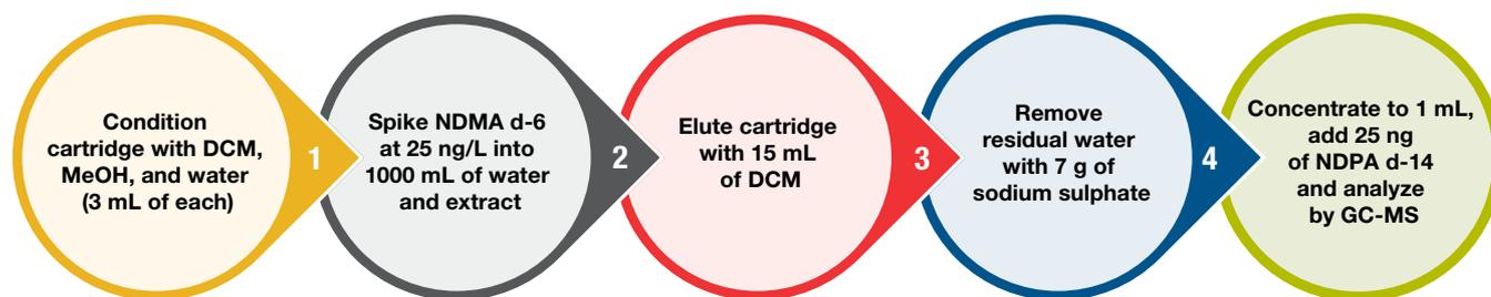
Figure 1. SPE steps used for drinking water samples
