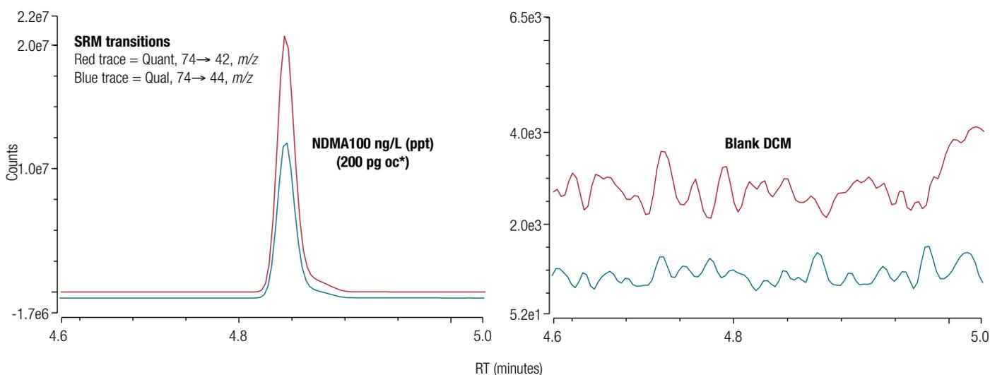
Figure 2. NDMA overlaid quantification ion and qualification ions for the highest standard in dichloromethane 100 pg/μL corresponding to 200 pg on-column (oc\*) (left chromatogram) and a consecutive DCM blank (right chromatogram). Data is unsmoothed and was acquired in timed-SRM mode.
