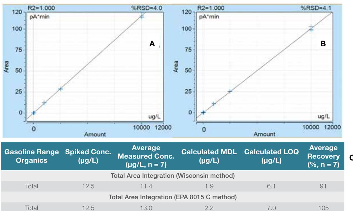
**Figure 3.** Calibration curves were obtained integrating the total area within the gasoline range at each calibration level for Wisconsin (A) and EPA 8015 C (B).  $R^2$ , response factor relative standard deviations (% RSD) as well as calculated MDL, LOQ, and percent recovery (C) are shown.
