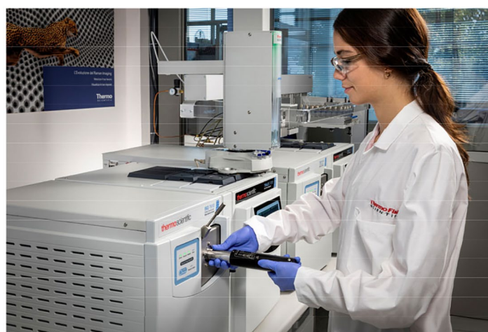
Figure 4. VPI being removed from the ISQ 7610 MS
