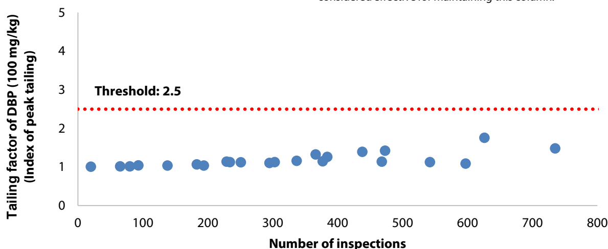
Fig. 2 Result of Evaluation of Durability in RoHS Inspections Using High Durability Column
