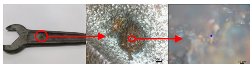
Fig. 10 Tool with Patch of Rust
