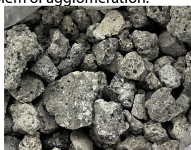
Fig. 1 Lumps Considered to Cause Agglomeration (Mixture of Gray and White Coarse Particles of Bottom Ash) (Long diameter: 2 cm to 5 cm)
