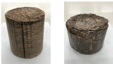
Fig. 2 Biocoke Produced from (Left) Waste Wood and (Right) Buckwheat Husks
