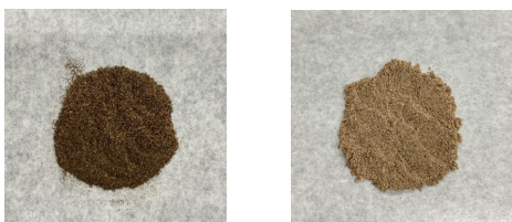
Fig. 3 (Left) Waste Wood and (Right) Buckwheat Husks after Screening with 250 μm Sieve
