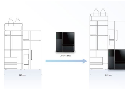
Figure 1. Integration of LCMS-2050 into an existing LC system.
