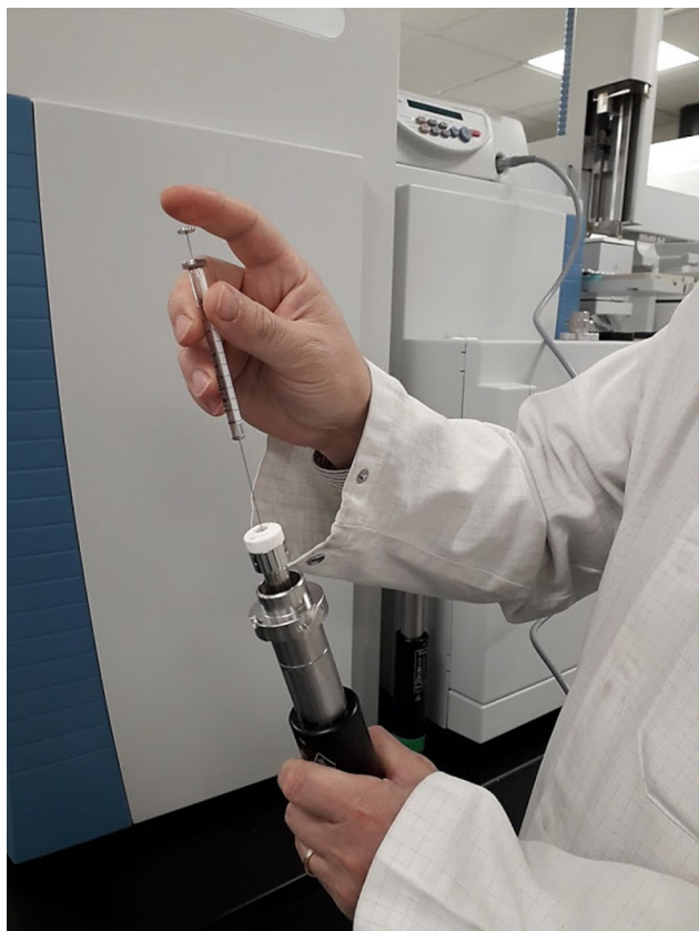
Figure 1. DIP sample loading procedure
