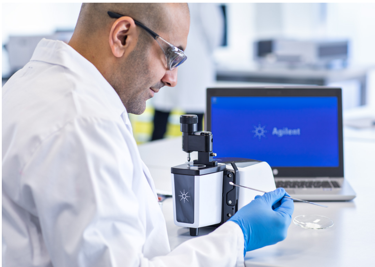
Figure 1. The Agilent Cary 630 FTIR spectrometer. With its ultra-compact design (footprint of 20 x 20 cm and weighing only 3.6 kg), the Cary 630 FTIR can easily be used where needed to produce high-quality results for incoming LIB raw materials.
