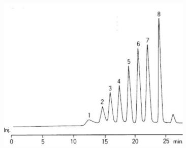
1. Polystyrene M.W. 9,120 K 2. Polystyrene 1,100 K 3. Polystyrene 410 K 4. Polystyrene 115 K 5. Polystyrene 33 K 6. Polystyrene 7.6 K 1.35 K 7. Polystyrene 8. *n*-Propylbenzene
