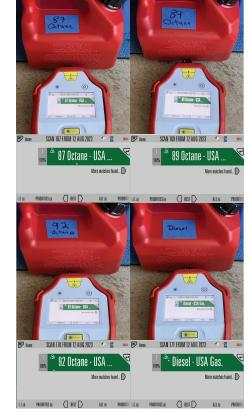
**Figure 6.** 100% match values for the four fuel sample measurements conducted through thick, red plastic containers using the Agilent Resolve and the custom "Fuels" library.
