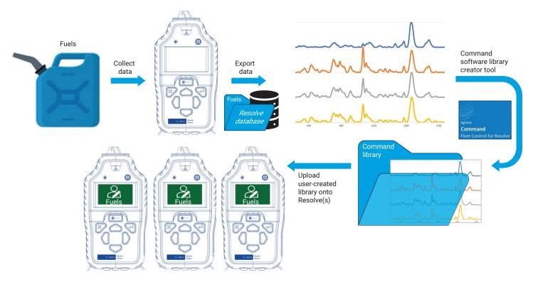
Figure 4. Workflow of data collection, library creation, and uploading of the user created fuel library from Agilent Command software to one or a fleet of Agilent Resolve handheld Raman analyzers.
