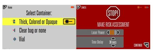
**Figure 1.** Left: Selection of Agilent Resolve handheld Raman analyzer operational mode; SORS through-barrier (Thick, Colored or Opaque), point-and-shoot (Clear bag or none), or glass vial measurements (Vial). Right: Risk assessment screen for reducing laser power or setting a scan delay time.
