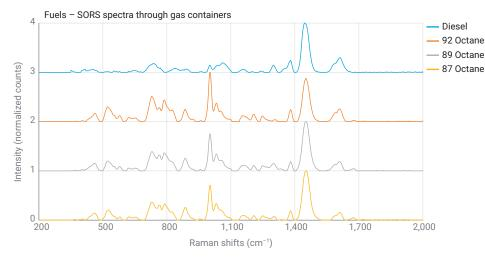
Figure 5. Raman spectra of four commercial fuels obtained using the Agilent Resolve handheld Raman analyzer in SORS through-barrier mode.
