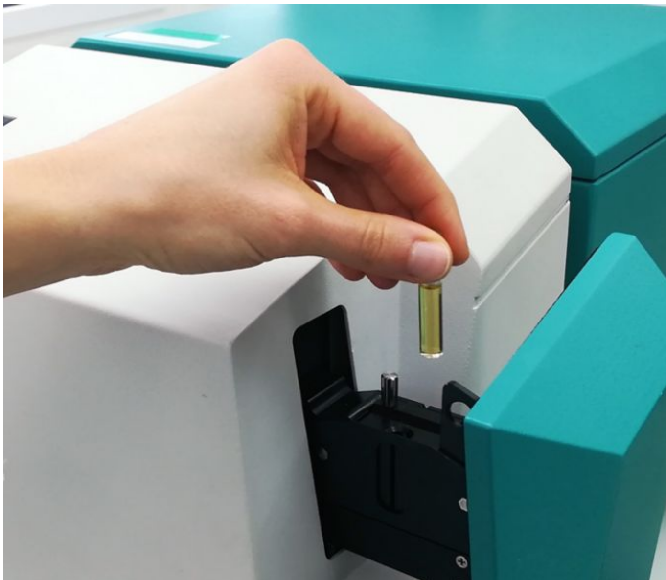
Figure 1. XDS RapidLiquid Analyzer and a polyol sample present in a 4 mm disposable vial.
