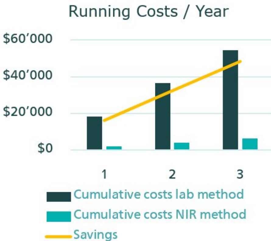
Figure 4. Comparison of the cumulative costs over three years for the determination of the hydroxyl number with titration and NIR spectroscopy.
