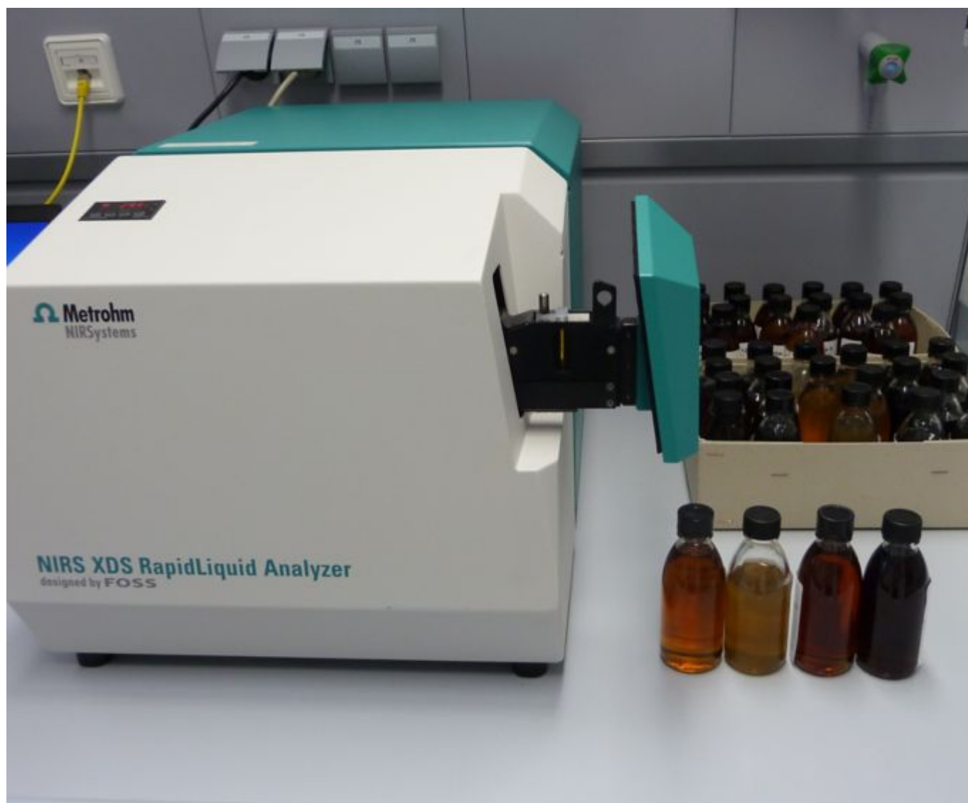
Figure 1. XDS RapidLiquid Analyzer and lubricant samples.
