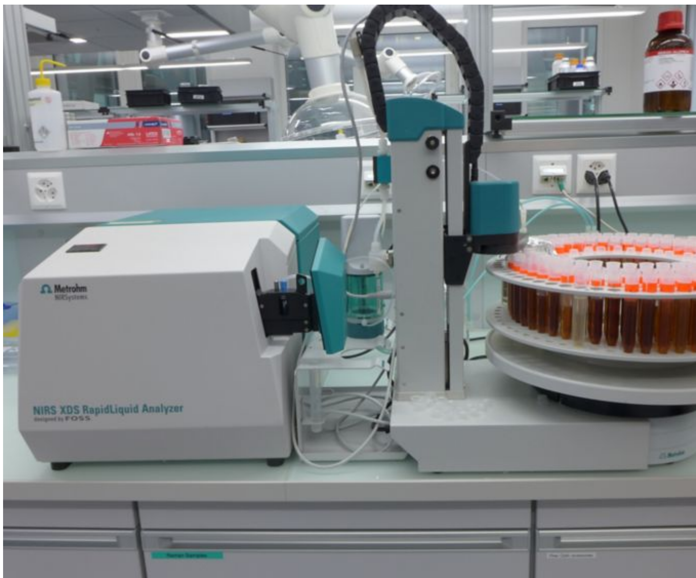
Figure 1. XDS RapidLiquid Analyzer with 5.0 mm flow cell and the 815 Sample Processor.
