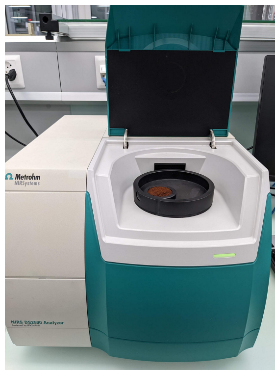
Figure 1. A Metrohm DS2500 Solid Analyzer with ground coffee beans held in a NIRS mini sample cup.
