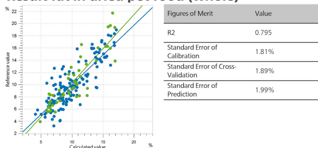
Figure 7. Correlation diagram and the respective FOMs for the prediction of fat in dried pet food (whole) using an OMNIS NIR Analyzer Solid. Blue dots represent calibration samples, green dots represent samples used to validate the model.
