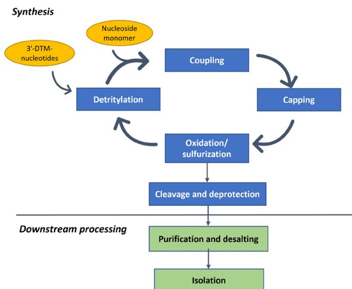
**Figure 1.** The oligonucleotide synthesis cycle and downstream processing steps.
