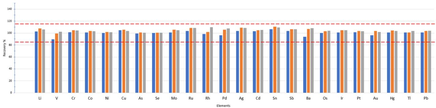
Figure 3. Accuracy results of spiked samples at 0.5 J (blue), 1 J (orange), and 1.5 J (grey).
