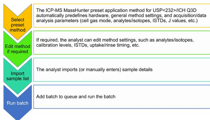
**Figure 2.** Method setup using the Agilent ICP-MS MassHunter Preset Method for ICH/USP elemental impurities.
