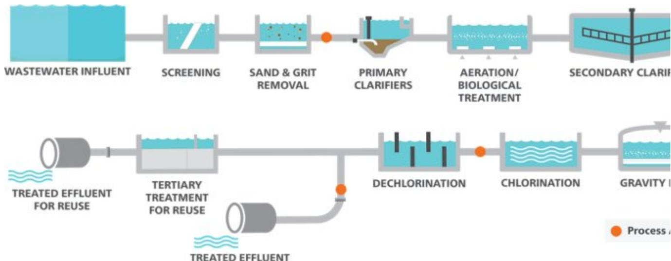
**Figure 1.** Process analyzer locations in the wastewater treatment process for phosphorus.
