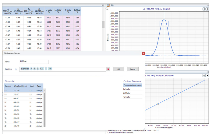
Figure 2. Using the custom column editing window in Agilent ICP Expert to convert quantitative results for La, Li, Ta, and Zr into molar percentages. The conversion is useful for reporting purposes.
