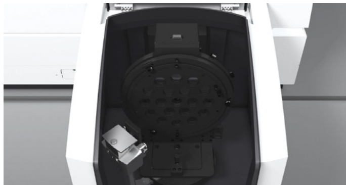
Figure 1a. Plan view of the Cary 7000 UMS measurement chamber with the Solids Autosampler installed.
