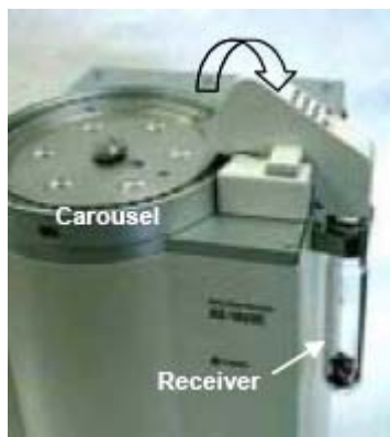
Fig. 4: Pyrolysis autosampler with carousel for 48 samples and cup receiver
