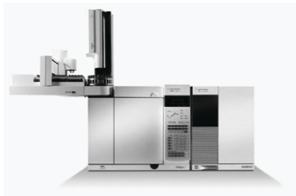
The Agilent 240 MS connected to the Agilent 7890 Series GC and the Agilent 7693 ALS.
