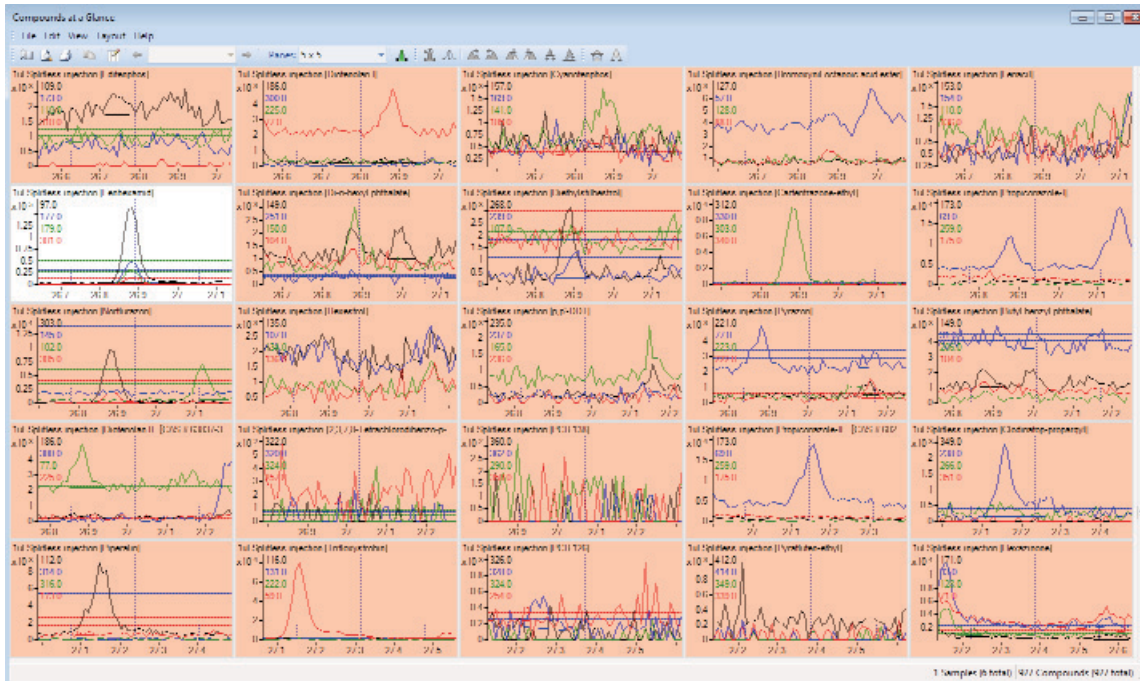
Figure 9. Compounds-at-a-Glance view. Target analytes failing one or more outlier tests are shaded in red.
